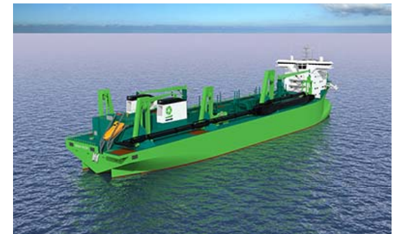
Bonny River - Trailing suction hopper dredger (14,500 m 3 )
