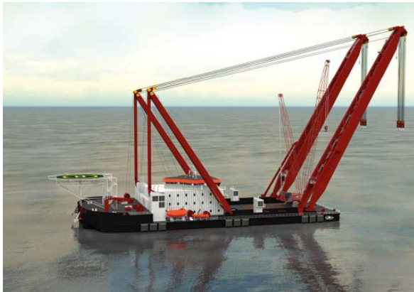
Gulliver Self-propelled crane ship (4,000 T)
