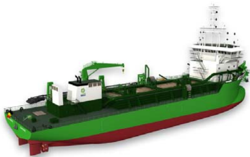
Minerva Hopper dredger (3,000 m 3 )
